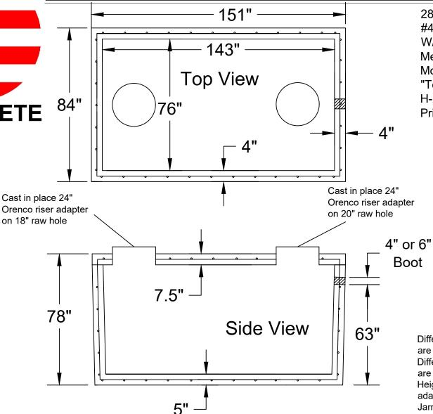
28 Day, 5,000 PSI Concrete #4 Rebar @12"o.c./e.w. Grade 60 W/ 6" Boots the Inverts Drops 1" Meets ATSM C-1227, 990, 923 Monolithic Tank Design "Top Tight" Patent Pending H-20 Traffic Rated Print Not To Scale
