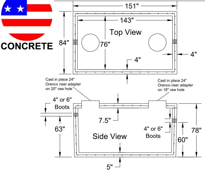
28 Day, 5,000 PSI Concrete #4 Rebar @12"o.c./e.w. Grade 60 W/ 6" Boots the Inverts Drops 1" Meets ATSM C-1227, 990, 923 Monolithic Tank Design "Top Tight" Patent Pending H-20 Traffic Rated Print Not To Scale
