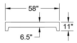
28 Day, 5,000 PSI Concrete G-60 #4 Rebar @ 12" o.c.e.w. Meets ASTM C-1227, 990, 923 H-20 Traffic Rated +/- 1/2" Tolerance
