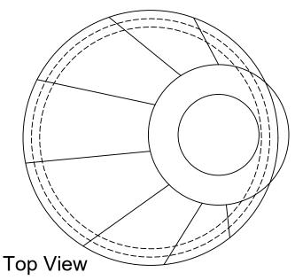
28 Day, 5,000 PSI Concrete #3 Rebar, Grade 60 Meets ATSM C-478 Steps As Required
