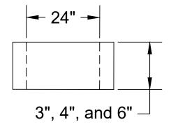
G-60 #4 Rebar @ 12" o.c.e.w. Meets ASTM C-1227, 990, 923 H-20 Traffic Rated +/- 1/2" Tolerance Print not to scale
