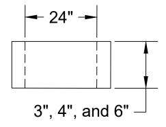
28 Day, 5,000 PSI Concrete G-60 #4 Rebar @ 12" o.c.e.w. Meets ASTM C-1227, 990, 923 H-20 Traffic Rated +/- 1/2" Tolerance **BASF 300D Admix** Print not to sclae
