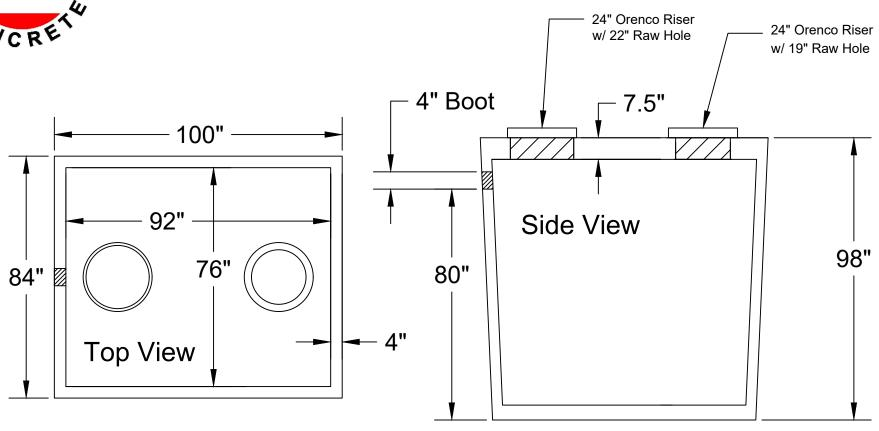
28 Day, 5,000 PSI Concrete G-60 #4 Rebar @ 12" o.c.e.w. Meets ASTM C-1227, 990, 923 Monolithic Tank Design "Top Tight" Patented H-20 Traffic Rated +/- 1/2" Tolerance
