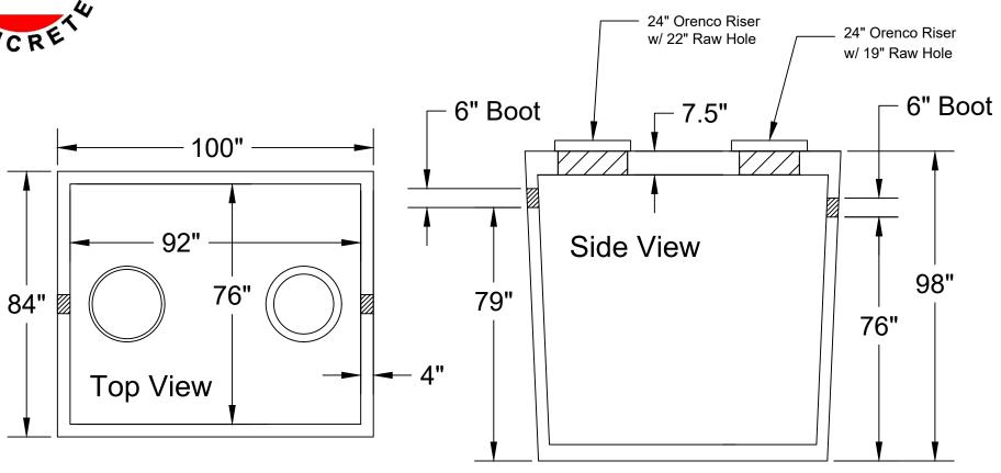
28 Day, 5,000 PSI Concrete G-60 #4 Rebar @ 12" o.c.e.w. Meets ASTM C-1227, 990, 923 Monolithic Tank Design "Top Tight" Patented May contain fiber in mix design Tank may be epoxy coated H-20 Traffic Rated +/- 1/2" Tolerance
