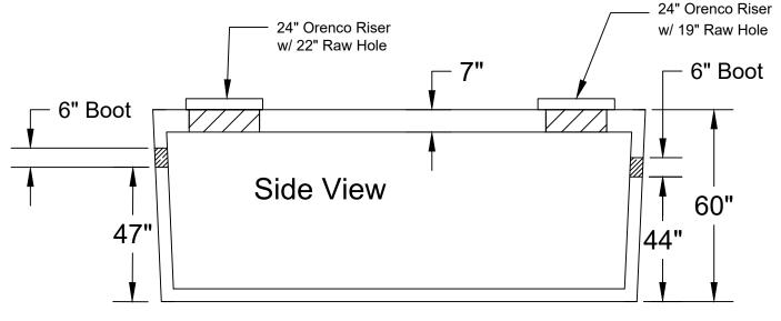
28 Day, 5,000 PSI Concrete G-60 #4 Rebar @ 12" o.c.e.w. Meets ASTM C-1227, 990, 923 Monolithic Tank Design "Top Tight" Patented May contain fiber in mix design Tank may be epoxy coated H-20 Traffic Rated +/- 1/2" Tolerance
