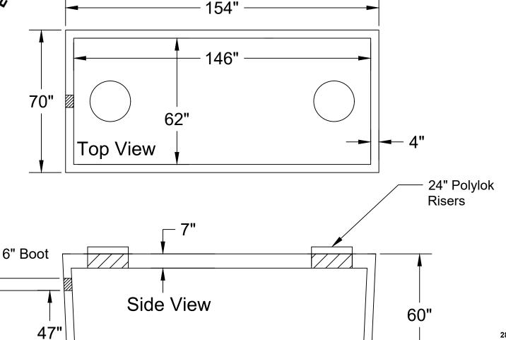
28 Day, 5,000 PSI Concrete G-60 #4 Rebar @ 12" o.c.e.w. Meets ASTM C-1227, 990, 923 **Monolithic Tank Design** "Top Tight" Patented May contain fiber in mix design Tank may be epoxy coated H-20 Traffic Rated +/- 1/2" Tolerance
