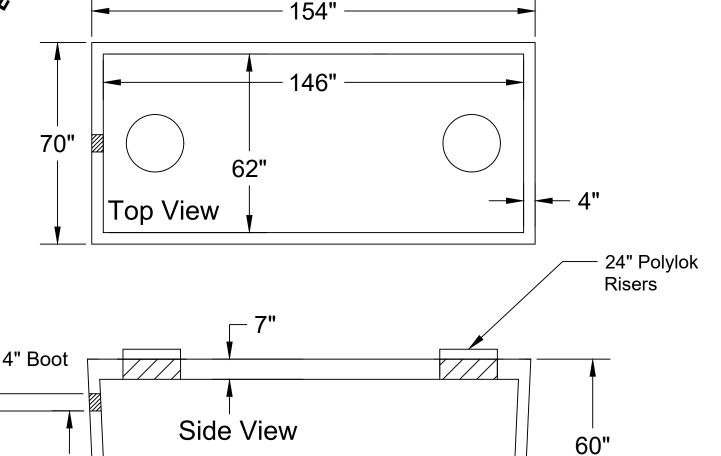
28 Day, 5,000 PSI Concrete G-60 #4 Rebar @ 12" o.c.e.w. Meets ASTM C-1227, 990, 923 Monolithic Tank Design "Top Tight" Patented May contain fiber in mix design Tank may be epoxy coated H-20 Traffic Rated +/- 1/2" Tolerance
