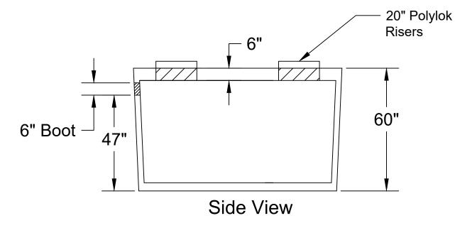
28 Day, 5,000 PSI Concrete G-60 #4 Rebar @ 12" o.c.e.w. Meets ASTM C-1227, 990, 923 **Monolithic Tank Design** "Top Tight" Patented May contain fiber in mix design Tank may be epoxy coated H-20 Traffic Rated +/- 1/2" Tolerance
