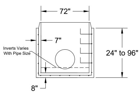
28 Day, 5,000 PSI Concrete G-60 #4 Rebar @ 12" o.c.e.w. Meets ASTM C-1227, 990, 923 H-20 Traffic Rated **BASF 300D Admix** +/- 1/2" Tolerance Print not to scale
