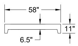
28 Day, 5,000 PSI Concrete G-60 #4 Rebar @ 12" o.c.e.w. Meets ASTM C-1227, 990, 923 H-20 Traffic Rated BASF 300D Admix +/- 1/2" Tolerance Print not to scale
