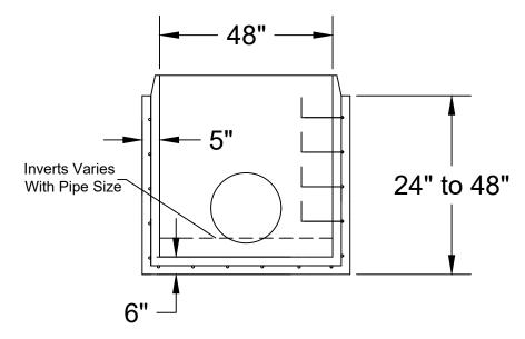
28 Day, 5,000 PSI Concrete G-60 #4 Rebar @ 12" o.c.e.w. Meets ASTM C-1227, 990, 923 H-20 Traffic Rated **BASF 300D Admix** +/- 1/2" Tolerance Print not to scale
