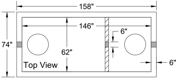
28 Day, 5,000 PSI Concrete G-60 #4 Rebar @ 12" o.c.e.w. Meets ASTM C-1227, 990, 923 Monolithic Tank Design "Top Tight" Patented May contain fiber in mix design Tank may be epoxy coated H-20 Traffic Rated +/- 1/2" Tolerance
