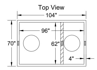
28 Day, 5,000 PSI Concrete G-60 #4 Rebar @ 12" o.c.e.w. Meets ASTM C-1227, 990, 923 Monolithic Tank Design "Top Tight" Patented May contain fiber in mix design Tank may be epoxy coated H-20 Traffic Rated +/- 1/2" Tolerance
