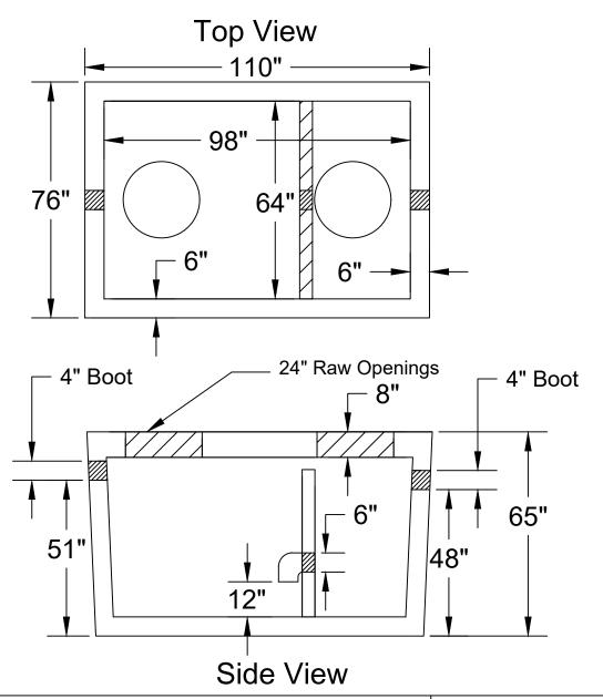
28 Day, 5,000 PSI Concrete G-60 #4 Rebar @ 12" o.c.e.w. Meets ASTM C-1227, 990, 923 **Monolithic Tank Design** "Top Tight" Patented May contain fiber in mix design Tank may be epoxy coated H-20 Traffic Rated +/- 1/2" Tolerance
