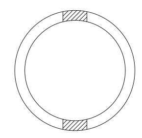
28 Day, 5,000 PSI Concrete G-60 #4 Rebar @ 12" o.c.e.w. Meets ASTM C-1227, 990, 923 H-20 Traffic Rated **BASF 300D Admix** +/- 1/2" Tolerance Print not to scale
