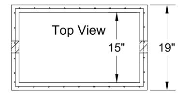
28 Day, 5,000 PSI Concrete #3 Rebar on 12" Centers Print Not To Scale
